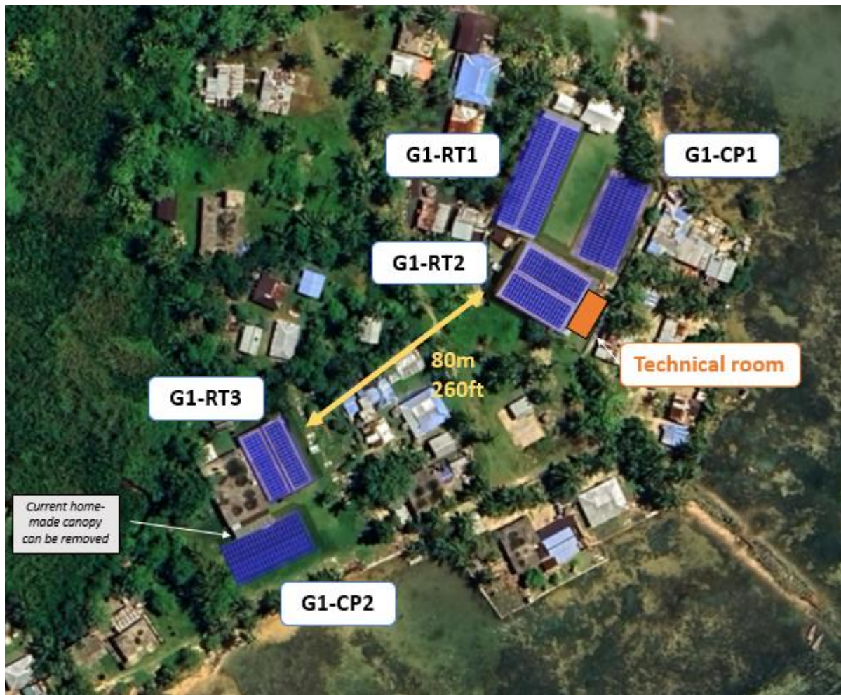
Figure 1. Top-view of PV array locations in G1
