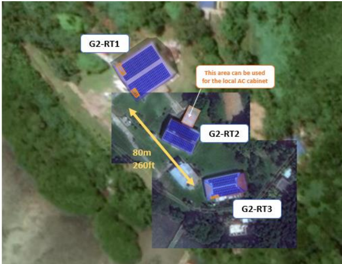
Figure 37. Top-view of PV array locations in G2
