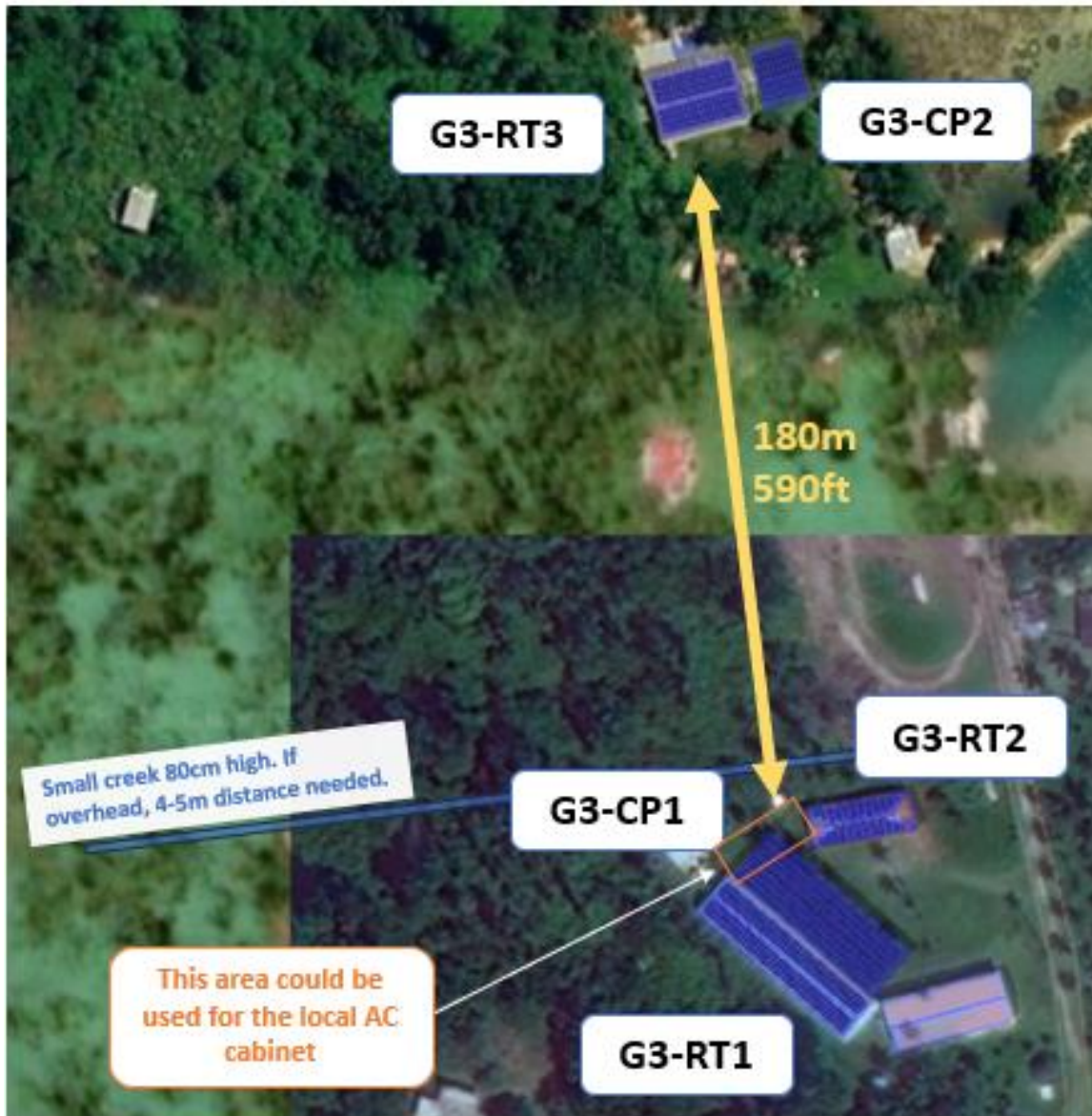
Figure 66. Top-view of PV array locations in G3
