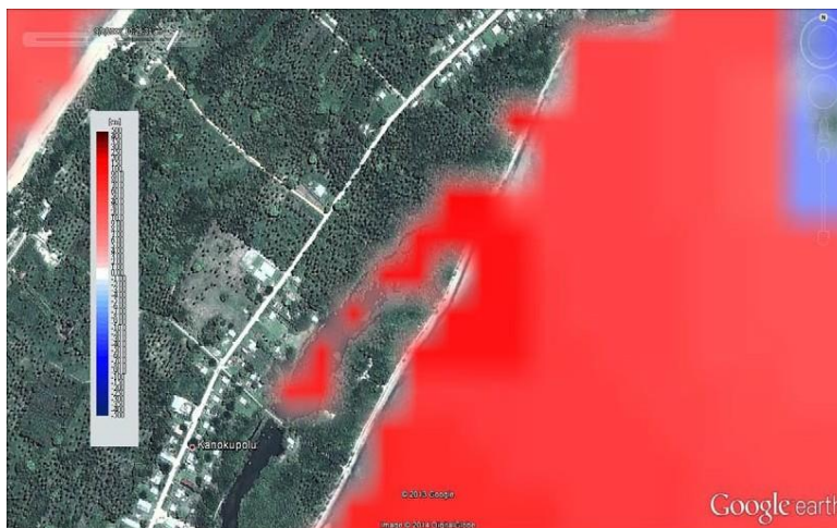
Figure 2-1. Close up of impact of a tsunami wave generated from an 8.7 magnitude earthquake at the Tonga Trench, showing two breaches of the coral foreshore (Geocare and Petroleum Consult, 2014).
